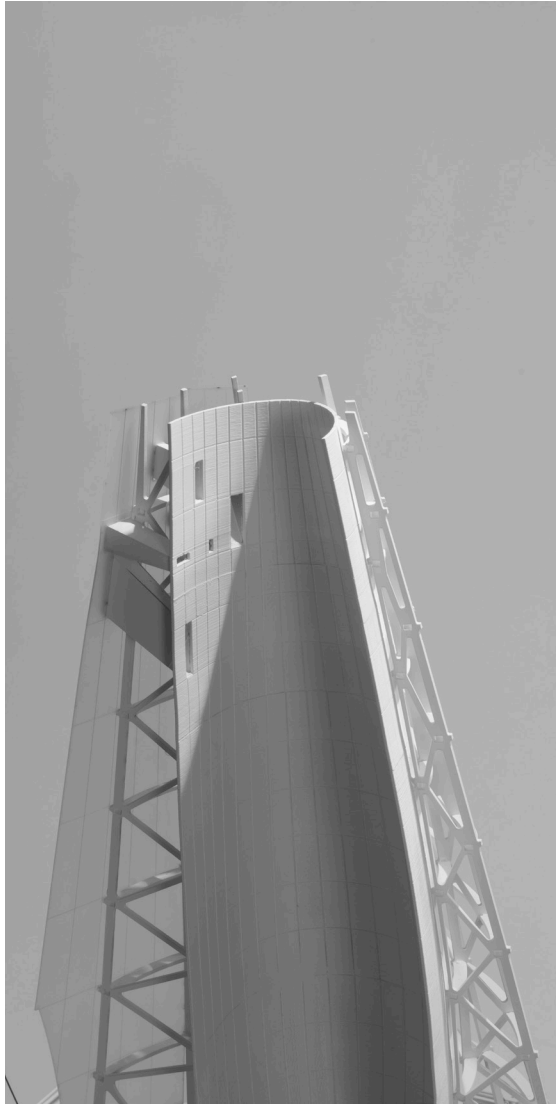
Overall structure model Resin, PLA, cardboard, music wire
